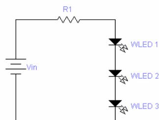
This topology can offer very high electric efficiencies (above 80%), especially when the total voltage drop across the LEDs array closely matches the power supply voltage. In this case a very small resistor is needed, where some power is wasted. Hence, virtually every watt consumed is used by the LEDs for the production of light. The design of a resistor-based LED driver circuit (LDC) comprises the following steps:
